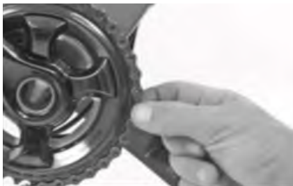
Check of the chain conditions.
