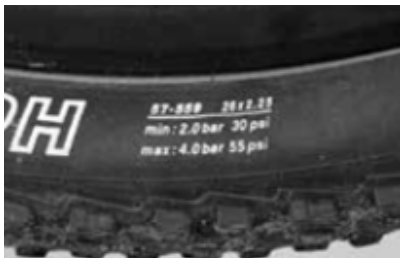
Sizes and pressure ranges of tire inflation.
